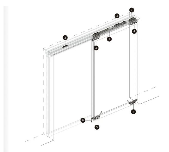
Install for top hung wheel Install belt holder
