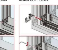
Install anti-rollback angle
