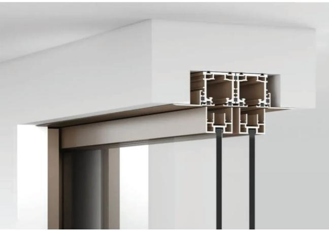
**SLIDING DOOR** FINISHED OPENING(FO) \*Inside door frame measurement **TOP VIEW** FO + 40mm = POCKET WIDTH FINISHED OPENING (FO) 30 mm POCKET WIDTH - 30 + FO = TRACK LENGTH (FO - 6 + 16)/2 = DOOR WIDTHDOOR PSS-A406 SYSTEM 6mm GLASS SEAL  $\triangle$  . DOOR PSS-A202-40 SYSTEM 40 DOOR FRAME(INNER) DOOR PSS-A203-40 SYSTEM 40 DOOR FRAME(OUTER) DOOR PSS-A403 BRUSH SEAL TRACK PSS-A328 SYSTEM POCKET ADJUSTABLE TRIM TRACK PSS-A363
